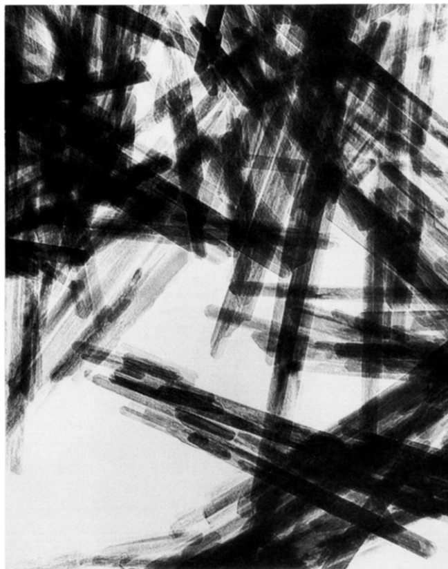
Figure 6. Transmission electron micrograph of OMS-2. Magnification is 380 000X.
